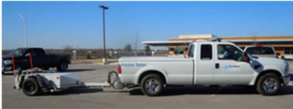
ARA's Austin-based locked wheel pavement friction tester
